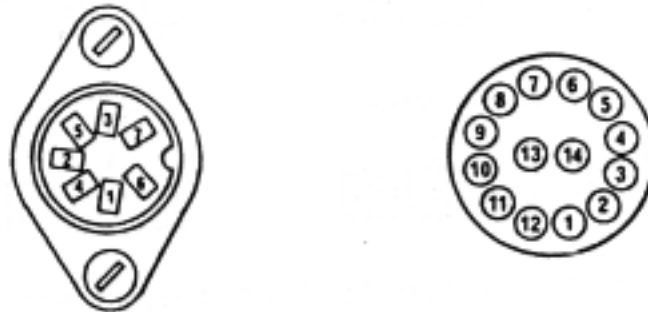
FIG. 9. REMOTE AND AUXILIARY SOCKET CONNECTIONS
