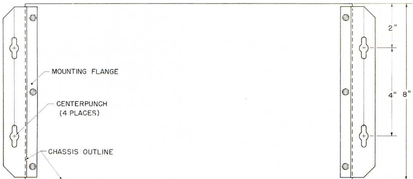
Figure 4. Bottom of MC75 with mounting flanges attached
