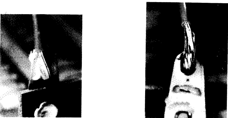
Fig. 7.8 Cold Solder Joint
