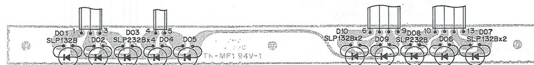
L.E.D. (SIGNAL) P.C.BOARD (BOTTOM VIEW)
